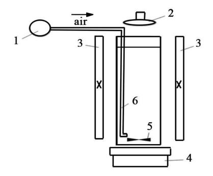
Fig.1. Schema of the photoreactor used for the cultivation of *Chlorella sorokiniana*: 1 – pump-aerator;
